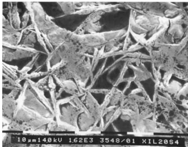
Figure 5 Scanning electron microscope analysis of sample film-XNC/X after 24 h of enzymic hydrolysis at 40°C.
